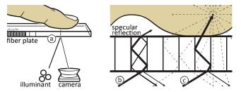
Figure 10: (a) The illuminant shines light onto the fiber optic plate. (b) A portion of the incoming light is reflected at the top of the fiber, traveling back down the fiber, where the camera
