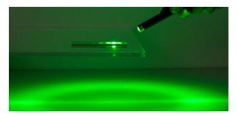
Figure 9: A fiber plate with a multitude of very small-diameter fibers (6μm) blurs ring diffusion, which scatters the incoming light into all directions. This is the basis for good light diffusion, which we need to produce an image on a touchscreen. The fiber plate rests 5cm above the table. The image on the plate is visible even from extreme angles.
