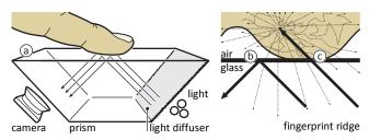
Figure 5: (a) Optical fingerprint scanners produce crisp contrast between fingerprint ridges and valleys using a prism. (b) Rays from the illuminant are totally reflected at the prism surface, causing such locations to appear *bright* as the camera sees directly into the light source. (c) Light escapes the prism (i.e., the reflection is frustrated) where fingerprint ridges touch the surface, causing ridges to appear *dark*.
