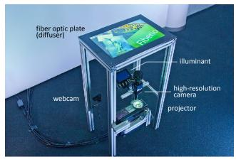
Figure 2: Our *Fiberio* prototype is a standard diffuse illumination setup, except that the diffuser is a fiber optic plate.
