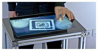
Figure 18: Fiberio recognizes touch, but also hovering objects (here fingers) as well as fiducial markers. The fiducial marker on this tangible object measures only 3mm×3mm.
