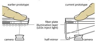
Figure 14: Fiberio evenly illuminates the entire surface, creating one even reflection to see fingerprints across the whole surface. (left) An earlier prototype used Acrylite LED below the fiber plate. (right) Our current prototype uses a half-mirror that reflects illuminations from the side.
