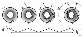
Figure 8: Each fiber diffuses parallel incident light into rings.
