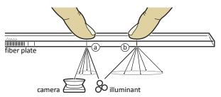
Figure 11: The light that comes back down the fiber is subject to same ring diffusion that we described earlier in terms of projection. While the camera will see reflections off the fiber plate's surface at location (a), reflections from location (b) will be invisible, because the camera does not sit on the same ring.
