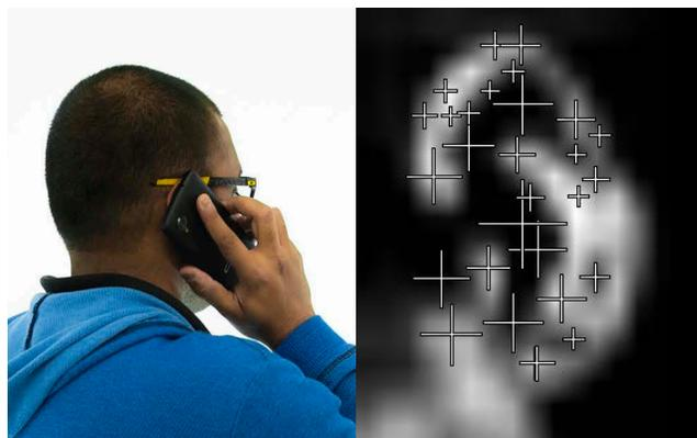
**Figure 1: *Bodyprint* brings biometric authentication to commodity mobile devices using the capacitive touchscreen as a low-resolution, but large-area image sensor to reliably identify users based on their ears, fists, or grips when pressed against the touchscreen. (left) To accept an incoming call, the user places the touchscreen onto his ear. (right) *Bodyprint* extracts features from the raw capacitive image to identify the user.**
