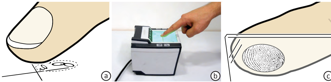
Figure 1.4: (a) Current touch devices infer input locations from the center of the 2D contact area between the user’s finger and the input surface. However, this causes them to record locations that are systematically offset from the target depending on the user’s finger pose (illustrated by the small ovals). We introduce the generalized perceived input point model , which models touch input on a per-user and per-finger-posture level to compensate for these offsets. (b) Our Ridgepad prototype is a high-precision touch-input device based on a fingerprint scanner. (c) Ridgepad implements our new model by identifying the user upon touch based on their fingerprint, and reconstructs the user’s 3D finger posture to make 2D touch more accurate.
