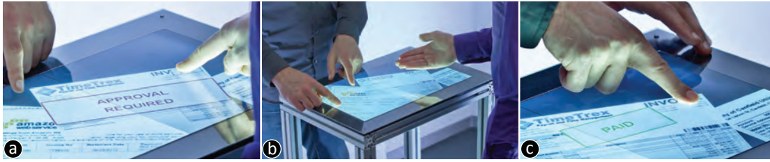
Figure 5.17: Example scenario. A bank manager (left) and clerk (right) approve invoices. (a) When the clerk encounters a bill above his approval limit, Fiberio refuses the payment transaction. (c) The manager completes the transaction by pushing the same button, but this time, Fiberio executes the operation using the manager's credentials, verifies it against his approval limit, and completes the operation.
