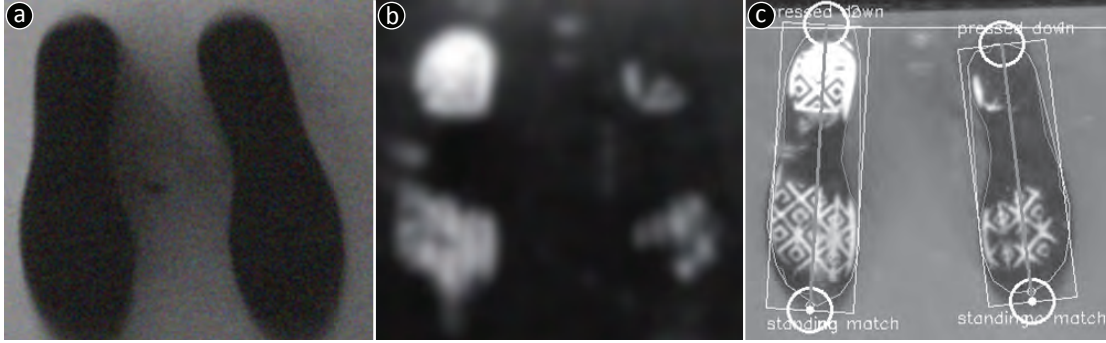
Figure 6.4: A user wearing shoes with black soles is standing on our floor prototype. (a) Front Diffused Illumination, (b) Frustrated Total Internal Reflection, (c) Front DI with FTIR, at 1 mm resolution camera.
