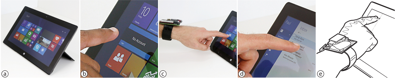
Figure 1: We enable commodity touchscreens to biometrically identify and authenticate users on every touch through the touchscreen itself. We seamlessly integrate continuous authentication into touch interaction, which fully replaces password dialogs.
