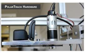
Figure 1. PolarTrack is an optical tracking system for mobile devices that combines an off-the-shelf RGB camera with a rotating linear polarization filter mounted in front of the lens. PolarTrack exploits the use of polarized light in current displays to segment device screens in the camera feed from the background by detecting periodical changes of display brightness while the linear polarizer rotates.
